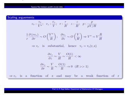
So we know that vertical velocity is of order V. So therefore we first normalize the axial velocity with V and then radial for the time being let us say it is V\* which we would like to estimate and then R is radius of the disk and z is normalized by the distance between the disks and pressure as usual which we have used okay. So now, let us consider our two terms in the equation of continuity.
