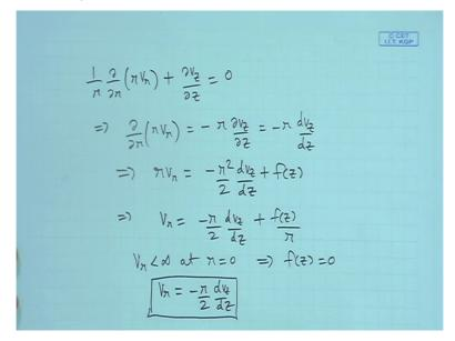
We have already seen this plus = 0 and then this vz is function of z, that already we have seen. So this implies -r so this I can write it as because its function of z alone. So now we integrate okay. So plus a function of z so this okay. But we need a boundedness condition. So that is Vr is finite at r = 0. So this indicates so therefore what we get is simply.
