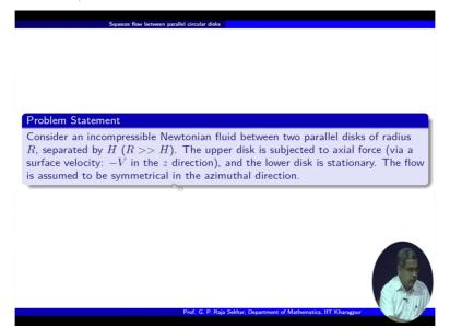
So the problem is we consider incompressible Newtonian fluid between two parallel disk of radius R separated by a distance H and we are assuming that R is much larger than H and as already indicated the upper disk is subjected to axial force. So typically when we say vertical so it is positive direction since we are pressing the disc so it is a taken away and negative okay.
