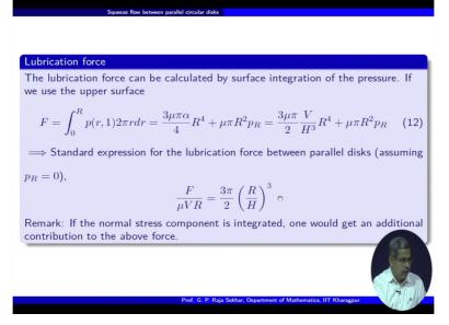
So this is called lubrication force and this can be calculated. So we are computing between 0 to R and at H equals to 1 considering H equals to 1. So we are integrating the pressure the corresponding areal element, then we have substituted p(r,1) okay that is computed. So then
