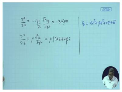
So we have the r momentum equation which is reduced already so that is okay. And we have vz structure here which is vz is written as Alpha z3 + Beta z power 2 + Gamma z + Delta okay. So therefore if we use three times okay so what we are going to get? This will be -3Alpha Mu r okay. So this one can just we have to compute third derivative substitute and we get this okay. Similarly we have okay.
