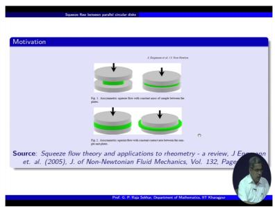
So there is some material and then you apply some force so then it gets squeezed it and then you get due to the corresponding flow you get the corresponding liquid like this okay. So there are a lot of applications so in particular filters and then some industrial dampers and where typically lubrication plays a vital role okay.
