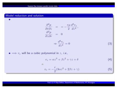
So from the z momentum equation we get this and for r momentum equation we get this? So in combining these two one can infer that the ODE for the vz is this. So this indicates the velocity structure will be a cubic in z. So where Alpha, Beta, Gamma, Delta, are some arbitrary constants that are to be determined. And once we have vz we can write down vr using the relation that we have okay.
