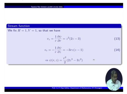
So we fix H = 1 and V = 1 just for the calculation purposes and then try to get the corresponding stream function okay. So vz is given by this and vr is given by this where Psi is a steam function and when we take H = 1 and V = 1, we get to the simplified expressions for the velocity components. So then one can integrate this to get the stream function okay. So the calculation is very straightforward so not explaining the integration.
