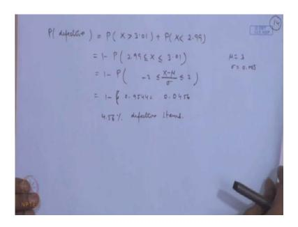
So, the proportion that will be declared defective that will be given by, that it is X is greater than 3.01 or X is less than 2.99 that is 1 minus probability 2.99 less than X less than 3.01. Now this you can shift to standard normal, here mu is equal to 3 and sigma is equal to 0.005.
