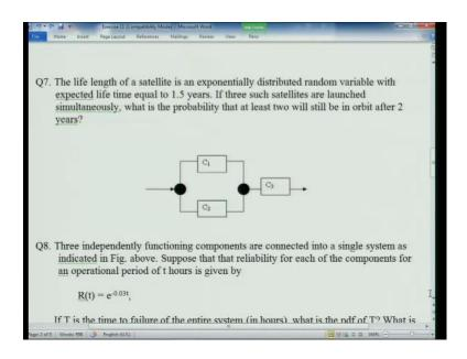
Now, this figure refers to problem 8, I think 3 independently functioning components are connected into a single system, as indicated in figure above. So, 2 are parallel and then 1 series, suppose that reliability for each of the components for an operational period of t hours is given by, e raise minus 0.03 t.
