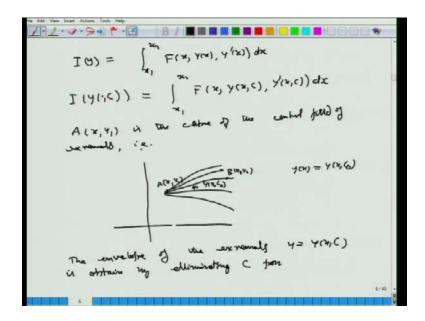
So we have this I(y)which is x 1 to x 2 f of x y x and y prime x d x. So, we consider here this I(y)on extremals only as before we considered only on the extremals, because; and this extremals should be an interior extremals like in this case this one it should not be boundary extremals. Like we have in the case of function the critical points are all those critical points are interior points not boundary points, boundary points minimum and maximum can occur in other ways also.
