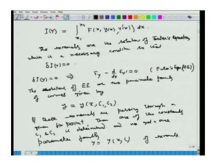
So, same manner we for the functional if we consider I (y) equal to x 1 to x 2 f of x, y (x), and y prime x. So, we see that like the points here of this equation, the extremals of the equation should be. So, the extremals are are the solutions of Euler's equation, which is obtained which is a necessary condition which is a necessary condition, so that this first variation delta I(y) equal to 0.
