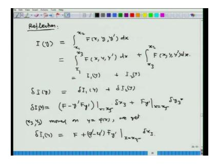
And so, we use the conditions here, this delta I which is some of these variations delta I 1 plus delta I 2, we break the integral x 1 to x 2 at x 3 which is the point x 3 y 3. And so, we get this delta I, evaluated at point x 3 minus that is a left limit and x 3 plus those in the 2 values are then equated.
