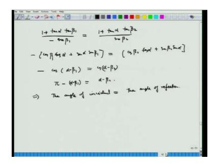
So, we got this condition here since these two angles are here beta 1 is like this and beta 2 is like this (Refer Slide Time: 04:24). So, we get here minus sign in this sec beta 1 here and then multiplying by cos beta 1 and the left side and cos beta 2 the right hand side, we get here, this minus cos of alpha minus beta 1 equal to cos of alpha minus beta 2. So, this is phi minus alpha minus beta 1 equal to alpha minus beta 2.
