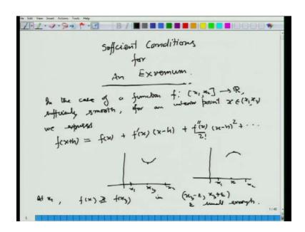
So, if f double prime is positive then we have minimum. So, if f double prime (x) is positive we have minimum, if f double prime (x) is negative then we have maximum, because in this case then you should have the situation like this. In the case of maximum the function should be like this at x 1, x that is why this is x 3 this is x 3. So, x 3 minus x 1 x 2 for the interval boundary points of the interval and x 3 is an interior point, so that is what should happen here.
