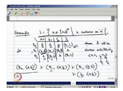
Say, this is an linear bounded automaton, which generates accepts all string containing an a. Any string containing a will be accepted by this linear bounded automaton, which is shown in that table the moves of the linear bounded automaton is shown in that table. So, q 0 q 1 q 2 order states of the linear bounded automaton a b are terminal symbols. And left angular bracket and right angular bracket are two special symbols that we have at left end marker, and right end marker.
