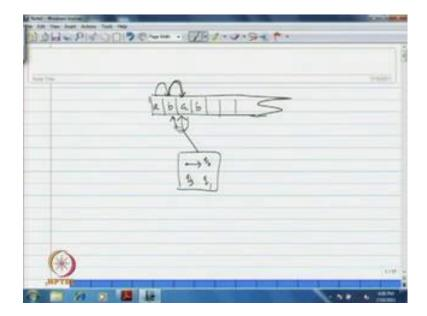
Like that we have in case of this two way finite automaton if you recollect, this thus schematic diagram of DFA or NFA, there you have input tape divided into two cells. And the input symbol that you are placing say like this and you have a finite control from which a reading and reading head connected to this input tape and there the state components that you have a pointer.
