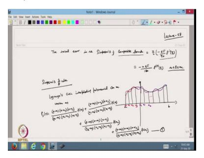
Now in the previous lecture the error, the total error in the Simpson one third for the composite formula, so that will be, because in this, in the previous case, in the Simpson one third rule, we apply the composite for n/2 times, so that is why instead of multiplying by n, we have to multiply by n/2 to the error, this one. So, this is the error for the Simpson one third rule and then I multiply it by n/2 because we are repeating this process n by 2 times.
