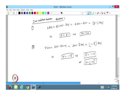
Now, we want to find the relations. So, I can define the other one: the interrelation between operators. So, what is the relation between the forward operator or the backward operator or the shift operator So, that we want to see. So, this is the interrelations between operators. So, suppose I want to display the first one I know that if I have the forward operator to the function at x, then it will be f(x + h) - f(x) and this one I can write as.
