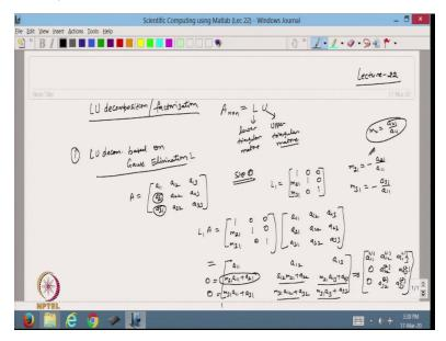
So, today we will discuss the next method and that is called LU decomposition or factorization. So, LU decomposition, so in this case what we are going to do? I have a matrix, so that is n\*n matrix, now I am going to decompose this matrix or factorize with this matrix into the LU form. So, where L is my lower triangular matrix and this U is upper triangular matrix.
