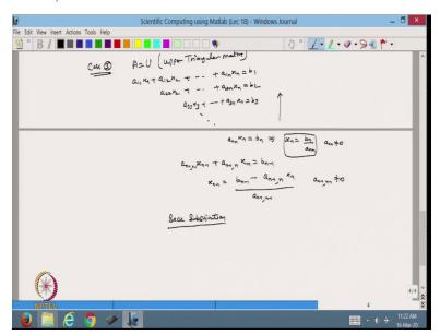
$$x_1 = \frac{\left(b_1 - \sum_{j=2}^n a_{1j} x_j\right)}{a_{11}}, \ldots, x_{n-1} = \frac{\left(b_{n-1} - a_{n-1,n} x_n\right)}{a_{n-1,n-1}}, x_n = \frac{b_n}{a_{nn}}.$$
