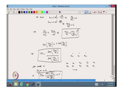
So this is how to find convergence rate numerically. Like suppose we made the code for Newton Raphson for the fixed point for the Regula-Falsi so in all the cases we will want to see how we can find the rate of convergence numerically. So, how we will do:
