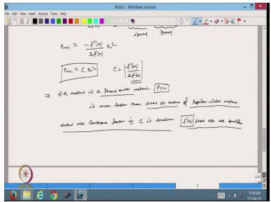
Then we have to apply this condition also that if this condition is satisfied only then my Newton Raphson method will converge and if it converges then definitely faster order. So, based on this one I can say so the method will converge faster if c is smaller because as small the c is the error will be reduced in the next step and the method will be much faster.
