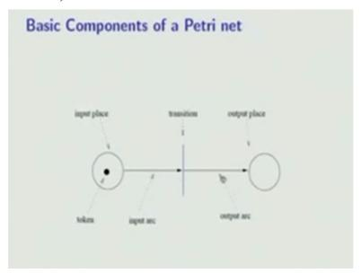
See this diagram, here are the basic components of a petri net. This is called input place and this arc is called input arc because the arc is connecting from the place to transition and this is called, the line is called, the bar is called a transition. The transition with the place that arc is called a output arc and the corresponding place is called output place. The number of dots inside the place is called tokens. Here input place has one token whereas this place has no token.
