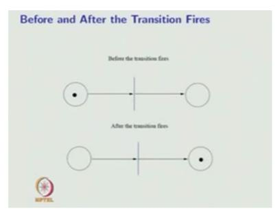
In the same example, before the transition fires, one token in the input place, no token in the output place. Whenever there is a token in the input place, then the condition is active. Then the transition first enabled, after the transition enabled it fires. After the transition fires the token will be removed from the input place and the token will be deposited to the output places.
