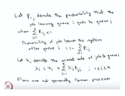
So in steady state whenever you have open queuing network with these assumptions in study state is this behaves as a independent queueing, therefore the joint probability of a n 1 customer in the first queue, n 2 customers in the second queue similarly and so on till the n k customers in the k th node, since each nodes behaves independently so the number of customers in different queues are independent.
