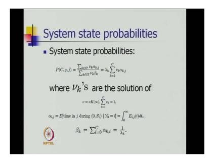
First you create the global kernel, then create the local kernel, then obtain the steady state probability vector V k's also find out the mean time alpha i comma j, using that we can find out steady state probabilities.
