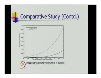
Similarly, as the rate increases because the X axis 1 divided by the mean handoff inter arrival time. Therefore, 1 divided by mean time is nothing but the rate. So, has the rate increases the dropping probability increases for the various distribution also. In this lecture, we have covered as a application of Markov regenerative process with the G M 1 N queue as well as the application of Markov regenerative process in performance analysis of wireless networks.
