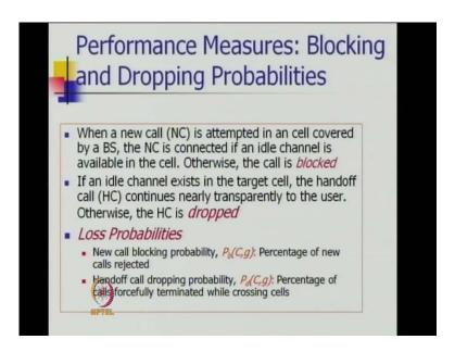
Similarly, the handoff call dropping probability in a cell, that is denoted by P suffix d. It is a function of C with the G, that is nothing but the percentage of calls forcefully terminated while crossing cells. So, here we are finding the two last probabilities, one is new call blocking probabilities and other one is handoff call dropping probability. In
