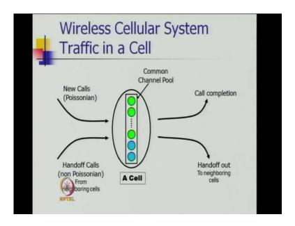
So the new calls follows the new call arrival follows Poisson process where as a the inter arrival of handoff calls follows general distribution and totally we have capital C channels out of that g channels are got channels which is reserved for.
