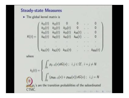
So, suppose the system start from the state n the p of n comma j of t is nothing but what is the probability that the system will be in the state j at time p given that it was in the state n at time 0. So, the previous explained the p i comma j are the transition probability of the subordinated CTMC. So, you need for all values of i and j and you have to find out the transition probability from these subordinated CTMC.
