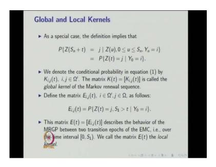
To study the limiting behavior first, we need the global kernel k of t it is consist of a matrix elements K i j of t and the another matrix local kernel that is the matrix E of t that consist of elements E i j of t, where i is belonging to omega dash, j belonging to omega.
