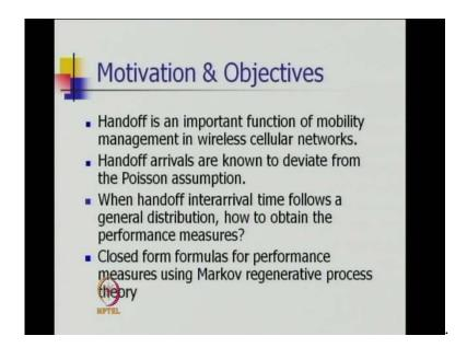
Here we are considering the handoffs in wireless cellular networks, what is the meaning of handoffs whenever the mobile station moves across a cell boundary, the channel in the old base station is a released and idle channel is required in the new base station. This process is called the handoffs process and corresponding calls are called a handoffs calls.
