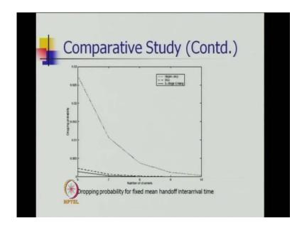
Similarly, you can numerically in the state the dropping probabilities versus number of channels are the different distributions for handoff inter arrival times with the fixed mean handoff inter arrival time.
