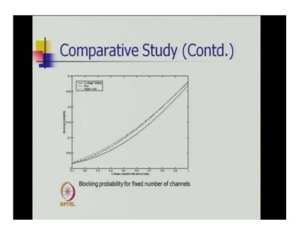
We can, we can illustrate the blocking probabilities versus the 1 divided by mean handoff inter arrival time. Also that means this the rate, so as the rate increases the blocking probabilities increases. The rate of handoff inter arrival increases the blocking probability increases for the various distributions.
