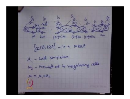
So, here is nothing but what is the probability that in a long run, the system is in the state 0 to in the state c minus g to c; that is the, that is the probability, sorry so the percentage of new calls are rejected will be the new call blocking probability.
