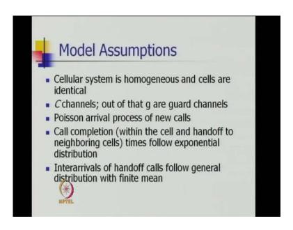
So here we make the assumptions for the cellular systems, the cellular system is homogeneous and cells are identical and assume that it has a capital C channels out of that g channels are guard channels. These guard channels are reserved for handoff calls.
