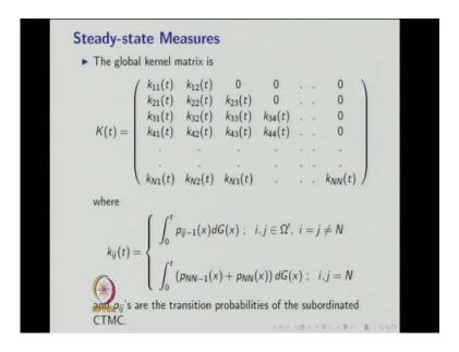
So, for this non Markovian queues we have a K of t matrix in this form with k i j of t is nothing but the integration between integration from 0 to t of p i j of p i j minus 1 of x integration with respect to G of x, where G of x is the c d f of inter arrival time. For i and j is equal to n will have a different expression. That means the system would have come from n minus 1 th the state to n th state or the system would have been stay in the same nth state retaining in the n of the state.
