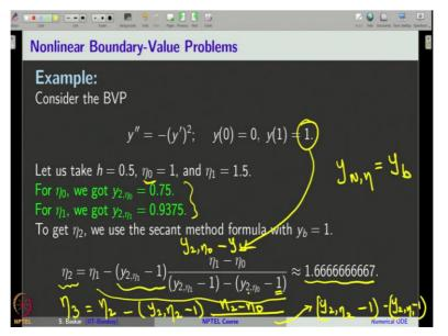
Let us illustrate the Shooting method with this simple non-linear ODE. We have  $y'' = -(y')^2$ . It is a non-linear ODE and we are given the boundary conditions as y(0) = 0 and y(1) = 1. Let us take h = 0.5 because we are going to do the computation manually. Therefore, it is better to take some big head h. So, that there is no much computation involved. To start with, we have to choose 2 initial guesses  $\eta_0$  and  $\eta_1$ , you can choose them arbitrarily.
