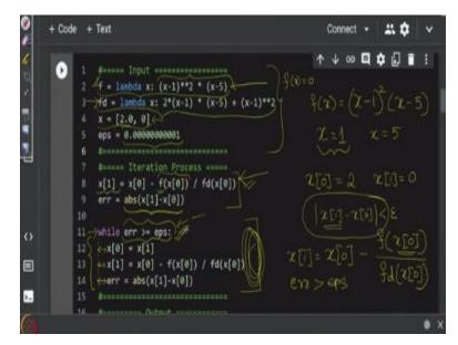
Let us start with the input. We have to take the function f which defines the equation f(x) = 0. And that is defined here, you can see that I am taking  $f(x) = (x - 1)^2(x - 5)$ . From this itself we can clearly see what are all the roots of the equation f(x) = 0. The roots are x = 1 and x = 5. The next thing is, we have to also input the expression for the derivative of f, that I am taking in the variable fd. Remember these two are going to be considered as exact expressions.
