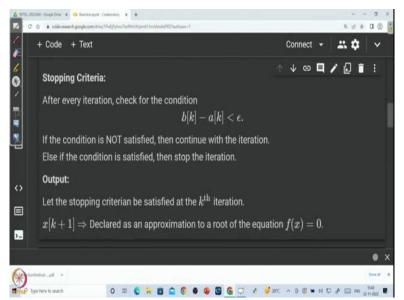
So, this is how we have built our algorithm in our previous class itself. I am just trying to recall it here. Now coming to the stopping criteria. We have to check whether b[k] - a[k] that is at every iteration. The length of the interval is less than  $\epsilon$  or not. If the length of the interval is
