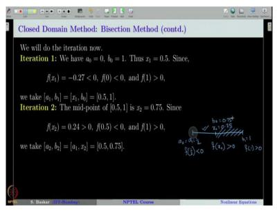
Let us go ahead and use bisection method for the given equation and compute three iterations and see how it goes. Well, for the first iteration, we have to give our interval  $a_0$  as 0 and  $b_0$  as 1. And now, for  $x_1$  we have to use the formula which is nothing but the midpoint of the interval [0, 1] that is nothing but 1/2. Now, we have to see whether the function *f* changes sign in this interval or in this interval.
