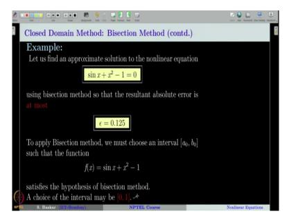
Let me take the interval as [0, 1]. You can check that f(0) is negative and f(1) is positive. Therefore, the interval [0, 1] can be a choice for our initial interval.
