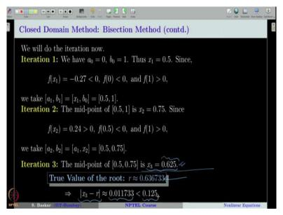
Let us go to the third iteration. You can see that the midpoint of the interval [0.5, 0.75] is given by 0.625 and that is it. We will stop here because we want the solution with accuracy, only 0.125 and our analysis says that you just have to carry three iterations. We have done the third iteration and take that value as the root. The problem ends here but let us cross check whether what our analysis says and what is the reality.
