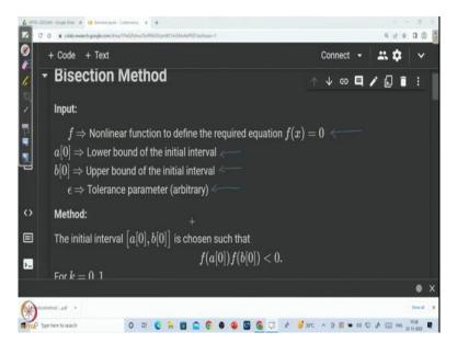
For that let us first see what are all the inputs needed for the code. Well, we need to give the function *f* that defines our equation f(x) = 0 and then we have to give the initial interval. For that we have to give  $a_0$  and  $b_0$ . Also, we will take the tolerance parameter  $\epsilon$ , that we will take as per our wish. There is no special property for  $\epsilon$  you can choose this arbitrarily.
