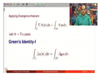
For some of them, we do not require all the hypothesis. So, now, if you apply a divergence theorem with psi = grad u, what we get is called Green's identity of 1. So, divergence of psi is now, divergence of grad u that is Laplacian u and grad u dot n is precisely the normal derivative of u dou n u, so, this is Green's identities one.
