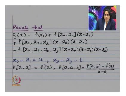
Now, let us recall that if  $x_0 x_1 x_2 x_3$  are distinct points then the interpolating polynomial  $p_3(x)$  is given by value of f at  $x_0$  plus divided difference of f based on  $x_0 x_1$  into x minus  $x_0$  then divided difference based on  $x_0 x_1 x_2$  into x minus  $x_0$  x minus  $x_1$  and the last term is divided differences based on the four interpolation points multiplications by x minus  $x_0$  x minus  $x_1$  x minus  $x_2$ .
