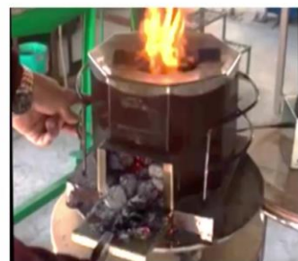
Fig.15 Demonstration of forced draft stove by the expert
