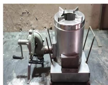
Fig.16. Eco Stove Designed and Developed for being distributed in the villages for household purposes
