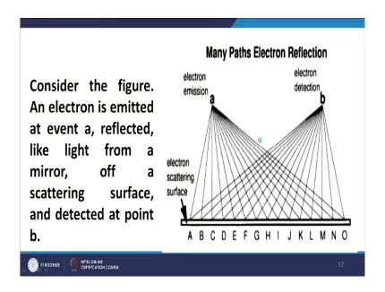
So, as an example let us consider this simple example. You have an electron which is emitted at the source a, it is reflected say by a magnetic, by a negative charge and mirror and it is identified or detected at the electron detector at the point b. So, for example, we have taken 15 different paths A B C D upto O.
