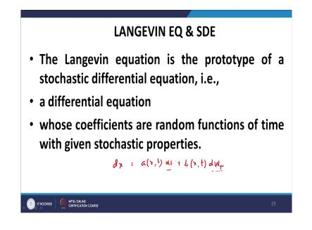
Now, the Langevin equation the which we saw just now V dot is equal to minus gamma V plus L t is a stochastic is an example of a stochastic differential equation. A stochastic differential equation is the differential equation where the coefficients of the various variables are random variables in themselves and they are also functions of time.
