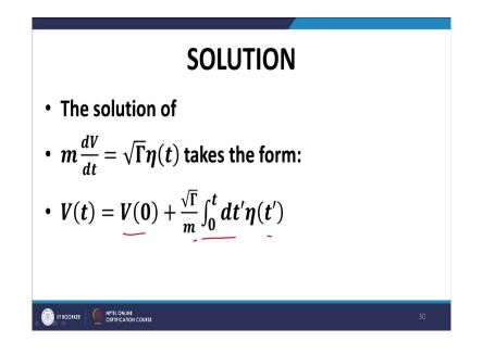
What is the solution of this equation? The solution of this equation is relatively straightforward. You can write it in the form V of t is equal to V 0 plus under root gamma upon m where, m is the mass of the particle in integral 0 to t dt dash eta t dash and so, this it is a straightforward see inhomogeneous first order equation. So, if we do not have much problem in writing down its solution.
