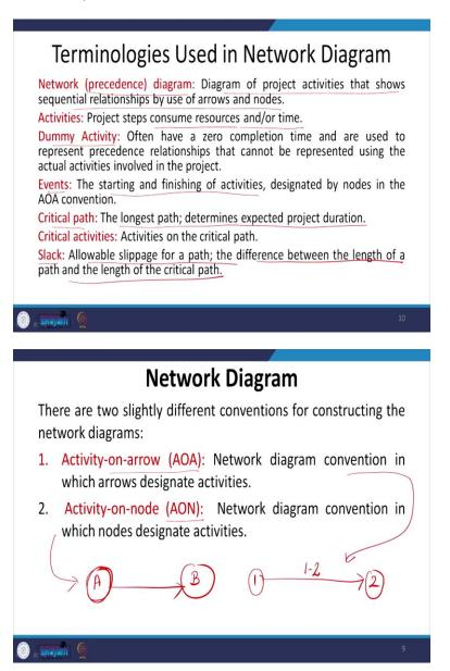
So, in the network or the precedence diagram as we understand the diagram of project activities that shows sequential relationships by use of arrows and nodes. So, two examples we just discussed AOA and AON. These are the ways in which we can represent our network diagrams.
