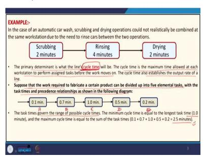
Now, with this simple example, you can understand the meaning of balancing. Now, we have 3 operations, scrubbing, rinsing and drying. Now, scrubbing takes 2 minutes, the rinsing takes 4 minutes and drying takes 2 minutes, so these 3 operations are taking different amount of time. Now, here you see the primary determinant is what is the line's cycle time. The first important thing is the cycle time determination.
