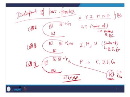
So, one of the important type of layout is cellular layout where the concept is like, we develop layout in the form of cells, we develop layout in the form of cells that different types of cells are generated and as I have written also that it is a type of layout in which work stations are grouped into cells. So, you have to develop cell.
