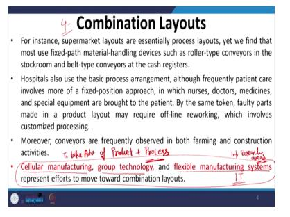
Now, the combination layouts are in a sense combination of product and process layouts. Now, here we have different type of names for the combination layouts, these are worth knowing that cellular manufacturing, group technology or flexible manufacturing systems, these are some of the very popular names, these are used very regularly whenever we are talking of advanced manufacturing techniques.
