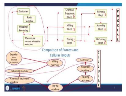
So, here you can have a very systematic comparison between your process and cellular layout. So, in this particular case if you see that there are different types of, this is the warehousing and that particular area where supply is coming. Now, here you have various processes, chemical treatment, milling, so you can name them as A, B, C, D, E, F.
