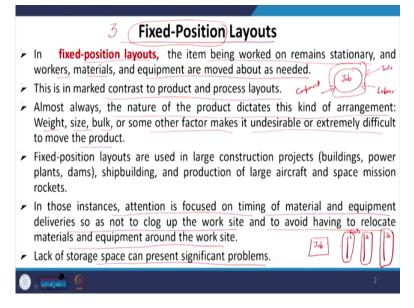
So now, another type of layout which is there, already two types of layout we have discussed, so this is the third type of layout that is fixed position layout. Now, fixed position layout and our earlier two layouts, the fundamental difference is that in that layouts our job, the work
