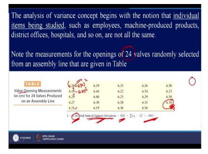
So let us say will take the valve opening example. So let us say there is something valve which has got the diameter like this right. So valves are being manufactured on 4 different machines right and let us say we have manufactured 24 valves and these are the diameters of these 24 valves. So let us say 6.26, 6.25 and so on right and the diameter of this valve is 6.34 right, so there are 24 valves okay.
