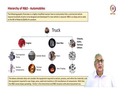
Let us look at an automobile. This illustrates in a highly simplified manner how an end product like a commercial vehicle requires hundreds of parts to be designed and developed if a new vehicle is required. R and D is as deep and as wide as the bill of material of a product. Bill of material is nothing, but a listing in a hierarchical manner, all the components that are required to manufacture a product.
