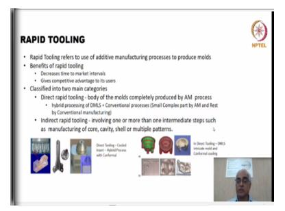
Coming to the tooling, so tooling is another big area where additive can play a big role. The reason why the tooling application is very wide for additive manufacturing is. The tooling is not getting into the final product, so we do not have to we can keep the tooling design in mind come considering the overall product application and then there is no need for any additional qualification or certification of the tooling itself.
