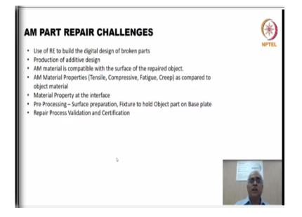
What are the challenges for the part repair using additive manufacturing? There are still process gets involved and then validated and then it is deployed. Few challenges which typically you come across while using additive as the process for part repair are, we need to build the model through reverse engineering, so that is the key thing to capture all the details and that is sometimes it may create an issue in while building the part.
