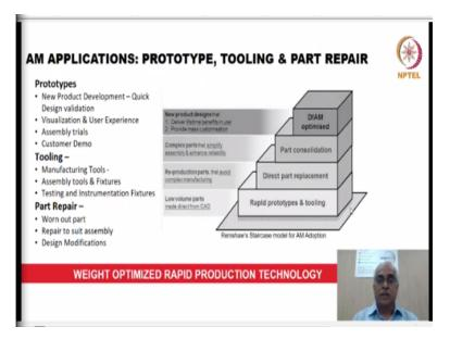
This has been one of the key areas where additive manufacturing has been widely used. In fact, that is what I like this staircase model from Renishaw which shows that at the bottom we have the rapid prototyping tooling. That is where the application of additive manufacturing started way back and with the lot of improvements which are happened in the metal printing.
