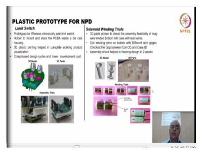
So, in many cases we do not make the prototypes for the actual material, we can make it out of polymers or plastics. So, there are some examples which I am showing it here. On the right-hand side, you can see that this is for the solenoid. The coil winding is the critical thing for the solenoid. We can do the winding trails on the bobbin of a polymer bobbin and then do all your winding trails and then finalize it and then reproduce that on the final part also.
