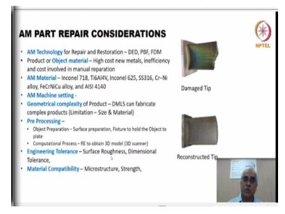
So, what we need to consider while we decide AM for the part repair ? One is we need to decide which technology you are going to use it for repairing whether it is a powder bed fusion or the FDM or the direct energy deposition. So, that depends on the type of repair what you want to do and then what capabilities each of these AM things offer today.
