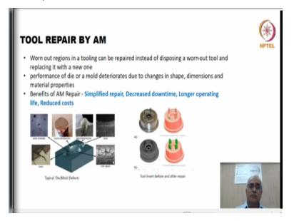
So, but nevertheless additive has been now very extensively used for many of the part repair activities especially the worn-out parts may not be the safety critical parts that in all other ideas been very widely used. You can see the type of defects which you can see in a dye and a mould in the picture. So, those are the defects which we can repair it using the additive manufacturing and then fix it.
