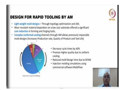
So, since we are using additive for these toolings we can take benefit of this additive. This is a typical application for the conformal cooling applications. So, when we do the mould designs, we always keep in mind how that mould can be produced. With the conventional of machining we can always have the straight, vertical or the horizontal or the holes we cannot have the curved holes.
