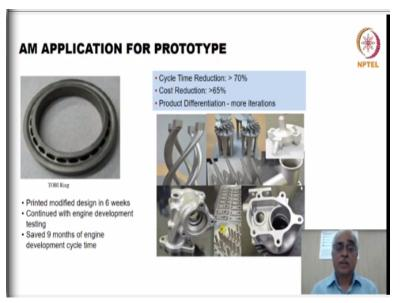
The next one is the TOBI nozzles. TOBI nozzles are the tangential injection of the cooling flow on the turbine blades to at the right pressure and temperatures, so that is a criticality of these TOBI nozzle designs. We could quickly get these things manufactured through the additive and we can take it to the testing. So, the one which is printed through additive may not have the life what we are looking at. But we can take it to the next assembly like engine testing.
