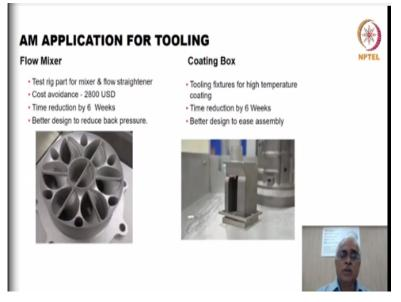
So, few more examples of the tooling here. This is a flow mixer; this is a test rig part for testing some of the flow meters or any other flow devices. So, this one we can come out with a real innovative design using the additive manufacturing by which we can reduce the cost. We can also reduce some of the back pressures which otherwise will be there with the conventional designs.
