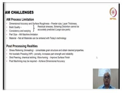
There are quite still a few challenges with additive manufacturing technology. These challenges could be in terms of achieving the final accuracy, dimensional accuracies, geometrical tolerances, the surface roughness. All this is decided by the powder size, the quality of the powder, the layer thickness. So, it still needs some sort of a post processing to address the final finish. But still it could be done much faster than the conventional but there are with these limitations still exist.
