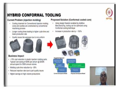
This is a practical example of deploying the hybrid conformal cooling. This is for one of the fire safety devices what we are talking about. The mould design was optimized by using the mould flow software and we could get a reduced cooling time of more than 50% as part of this. This design can see here that the conformal cooling which channels which are incorporated. So, that we can quickly cool the mould and then you also get the uniform temperature.
