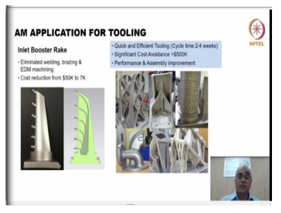
This is another good example of the rake, the measurement. It measures the pressure across the airfoil. Typically, this takes a lot of time to make it through the conventional process. It also involves a lot of welding, brazing and then the EDM machining if you follow the conventional process. Additive is the right way we can make this part and eliminate the welding, brazing which helps in reducing the cost as well as the cycle time.
