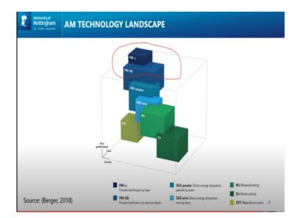
To answer this question, it is very important to understand the process landscape of additive manufacturing. Currently, additive manufacturing is currently in its formative phase and that is the phase between concept and growth of an innovation. This particular phase is characterized by lots of technological uncertainty and this is evidenced by the proliferation of different AM process systems in the marketplace.
