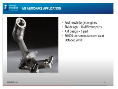
Another very good example from the aerospace is the fuel nozzle made by General Electric. This is a well cited application and in the same manner, the traditional manufacturer design consisted of 18 different parts. Those parts have now being consolidated into one with the capabilities of additive manufacturing. This has been a very successful application of 3D printing in the industry.
