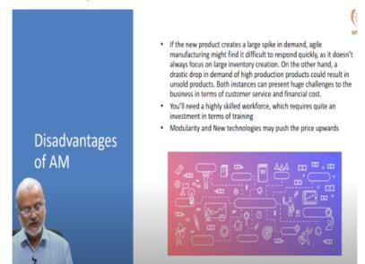
So, is it all good or all bit of roses for agile manufacturing? That we have to look at it. There is a specific time and situation for which again manufacturing can be applied. There are some disadvantages that are there, it is captured here. If the new product creates a large spike in demand, agile manufacturing might find it difficult to respond quickly.
