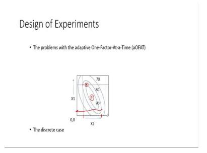
This is simple problem with that and we I am going to illustrate that with this diagram. Let us say that this plot that you has two input variables, input variable one x called  $x_1$  and input variable two called  $x_2$  and the output is nothing but, a hill that is projecting out
