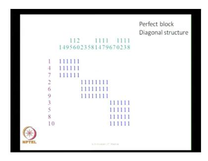
Now, this matrix has been specifically created so, that we get a very nice structure here, the second part of the algorithm which is actually identifying machine groups and part families from I a given block diagonal structure is very simple in this particular structure because which very evident that there are 3 groups now we see all the ones are clustered beautifully together there are 3 distinct blocks all the zeros are outside of the blocks.
