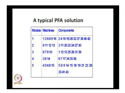
A typical PFA solution we have seen slide earlier in our example for the 16 machine forty 3 part example a typical PFA solution will be like this it will give the machines belonging to each group and components belonging to each group. So, the end of the production flow analysis algorithm we would get exactly how many groups we have what are the machines go to each group and what are the part are go to each group.
