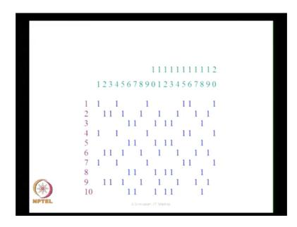
This is another example of a machine component incidence matrix this example has 10 rows and 20 columns which means 10 machines and 20 parts and components, if we carry out rank order clustering by doing it first for the rows and then for the columns we will get a structure like this.
