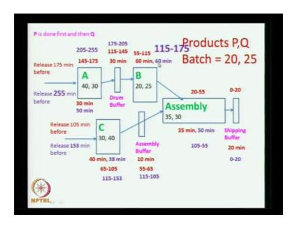
By now again advancing Q. So, Q is done between 115 and 175, P is going to be done later between 55 and 115. Now I move backwards drum buffer is 175 to 205 and A is 205 to 255. So, Q is released 255 minutes before. P retains 55 to 115, 115 to 145 drum buffer and 145 to 175 here.
