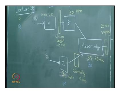
P has two raw materials R and S, R gets processed in A and B and goes to assembly. So, we will have 1 machine which is A, we have another machine B and then we have the assembly here we have a third machine C.
