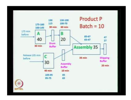
Now, this is how the next slide will look like. Now there are two ways of doing this computations, one is to start at 0 here at the end of the shipping buffer and then move backwards like we did in the previous slide. The other way is to start with 175 and 105 which were the numbers that we computed in the previous slide, and then move from left to right in the forward direction and see whether we are able to finish at 0 or whether we are able to finish before 0.
