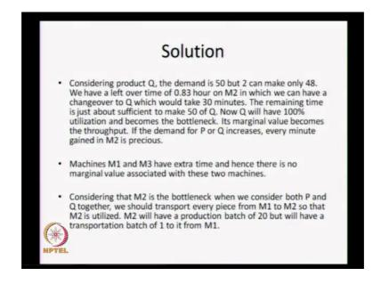
Which is what is shown in this bullet the demand is 50, but it can make only 48 we have a leftover time of 0.83 hour on M 2 which we can have a changeover which will take 30 minutes, Q will have 100 percent utilization and M 2 becomes the bottleneck. It is marginal value becomes the throughput and as demands increases every minute gained in M 2 is precious.
