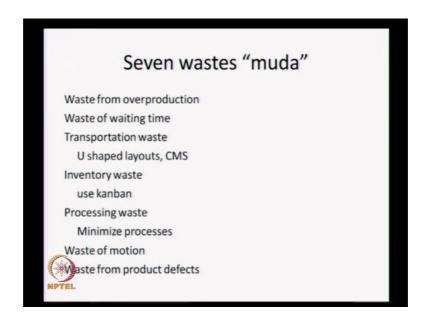
We have already seen that JIT is all about eliminating waste. So, we now look at how wastes can be classified. So, wastes are classified into seven distinct entities it is called seven wastes or 7 muda and these seven wastes are waste from overproduction, waste a waiting time, waste of transportation, waste of inventory, waste of processing, waste of motion and waste from product defects. So, these are the 7 wastes.
