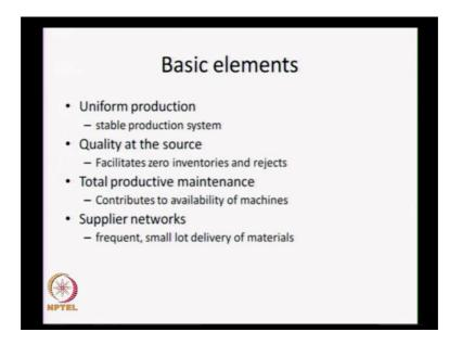
Uniform production also eliminates waste, uniform production is able to give a very stable production system and because the production is uniform and stabled there are less inventories of finished goods and once again this helps in eliminating wastes due to invented.
