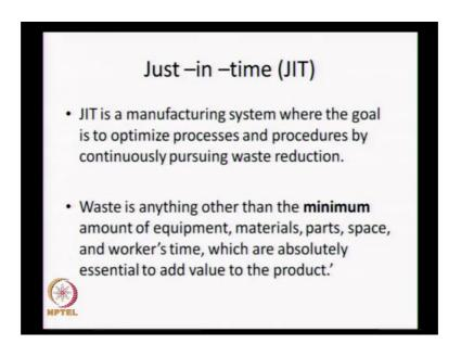
In the previous lectures, we have defined; what is just-in-time manufacturing. Just-intime is a manufacturing system where the goal is to optimize processes and procedures by continuously pursuing waste reduction. So, the main emphasis on JIT is waste reduction and waste is defined as anything other than the minimum amount of equipment, materials, part space and time which are absolutely essential to add value to the product. (Refer Slide Time: 00:53)
