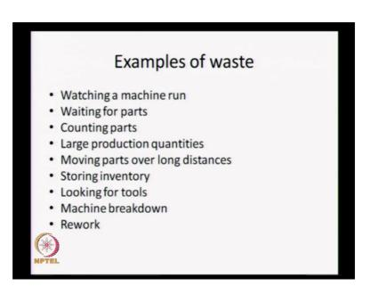
Watching a machine run, now watching a machine run becomes a waste because at this time when the machine is running and making a product the operator is not being utilized. So, the operator time is being wasted. So, this aspect we have seen in cellular manufacturing particularly when we have automatic machines how an operator can be assigned to multiple machines and the maximum of the operator time and the machine
