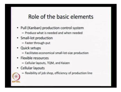
Now, what are the role of the basic elements? We have seen these basic elements here we spend a little more time on this. So, the pull system or a Kanban controlled production system, essentially eliminates waste by producing what is needed and then it is needed. So, we will see the role of the basic elements in terms of the fundamental principle of JIT that is to eliminate waste.
