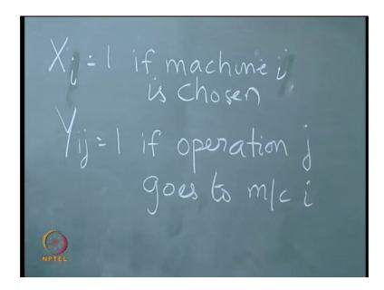
So, the formulation will become X j equal to 1 if machine j is chosen and Y or X i equal to 1 if machine i is chosen and Y i j equal to 1 if operation j goes to machine i. So, we have more variables that come in, and we if we have a cycle time restriction then we have to try and restrict the cycle time on each of these chosen machines and so on.
