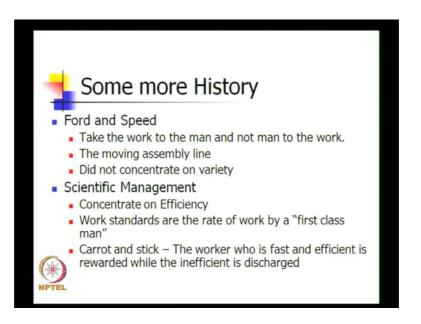
The next aspect that came into manufacturing was understanding speed now speed the emphasis of speed came from ford and the basic idea was to take the work to the man and not man to the work which resulted in the moving assembly line and there was not so much concentration on variety, but there was concentration on volume and speed of production.
