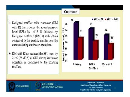
When the equipment comes in contact with the soil while being drawn behind the tractor what happens to that and, during that period, what is the load on the tractor and then what happens to the noise which we heard at the operators the ear level emanating from the exhaust of the engine? The cultivator (Refer Time: 30:59).
