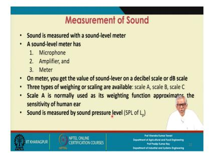
The sound is measured with a sound level meter. A sound level meter has three components. First one is the microphone, the second one is the amplifier and the third one is the meter.
