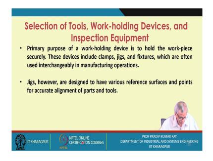
The primary purpose of a work-holding device is to hold the work-piece securely. These devices include clamps, jigs, and fixtures, which are often used interchangeably in manufacturing operations.
