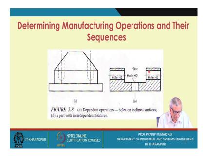
The second example is this is a slot to create. First you go for the drilling, and then you go for the milling operations.
