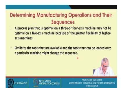
For example, a process plan that is optimal on a three-or four-axis machine may not be optimal on a five-axis machine because of the greater flexibility of higher-axis machines.
