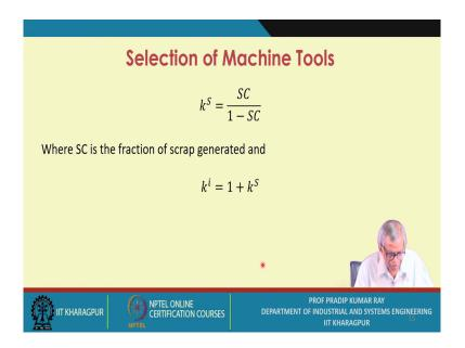
Because and you select that particular machine tool for which the amount of scrap is expected to be very less. So, and it has it must have sufficient capacity as well as the production rate.
