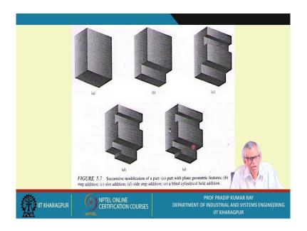
Now, this is an example from the textbook. (1) is part with the plane geometries; this one is actually the step and this is the slot and this is the additional step; that means, this is in the perfect raw form, then you start changing its shape.
