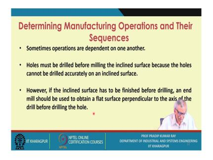
Sometimes operations are dependent on one another. I already have cited one example, milling versus the drilling, the holes must be drilled before milling the inclined surface, because the holes cannot be drilled accurately on an inclined surface.
