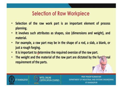
Selection of the raw work piece is an important element of process planning. It involves such attributes as shapes, size (dimensions and weight), and material. For example, a raw part may be in the shape of a rod, a slab, a blank, or just a rough forging. It is important to determine the required oversize of the raw part.
