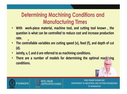
Having specified the work-piece material, machine tool, and cutting tool, the question is what can be controlled to reduce cost and increase production rate. The controllable variables are cutting speed (v), feed (f), and depth of cut (d). Jointly, v, f, and d are referred to as machining conditions. There are a number of models for determining the optimal machining conditions.
