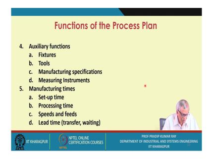
Then we will be referring to the auxiliary functions when you prepare this document, you will be always referring to not only the primary functions, but also the auxiliary functions such as the fixtures, tools, manufacturing specifications and measuring instruments. This is basically the work holding devices.
