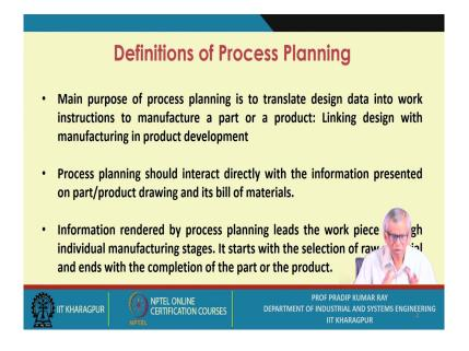
The main purpose of process planning is to translate design data into work instructions. The task of process planning is to translate design data to work instructions to produce a part or a product.
