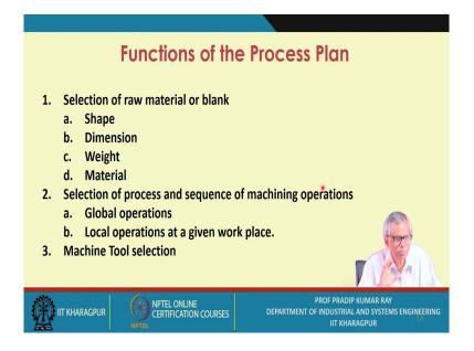
What are the functions of a process plan? First you have to select the raw materials depending on the type of part you produce. While you select the raw material, the shape of the raw material should be specified. These are the determining factors: the dimension, weight and the material.
