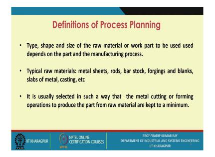
Type, shape and size of the raw material or work part to be used depends on the part and the manufacturing process. The form of the raw material used depends on the part and the manufacturing process. Typical materials are metal sheets, rods, bar stock, forgings and blanks or slabs of metal. It is usually designed such that the metal cutting or forming operations to produce the part are kept to a minimum.
