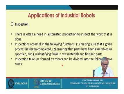
There is often a need in automated production to inspect the work that is done. Inspections accomplish the following functions: (1) making sure that a given process has been completed, (2) ensuring that parts have been assembled as specified, and (3) identifying flaws in raw materials and finished parts. Inspection tasks performed by robots can be divided into the following two cases:
