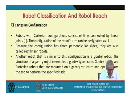
Robots with Cartesian configurations consist of links connected by linear joints (L). The configuration of the robot's arm can be designated as LLL.
