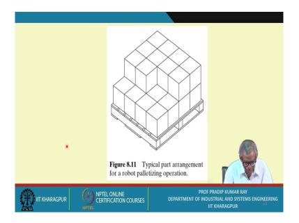
This is one problem, the typical part arrangement for a robot palletizing operation. All these parts are to be arranged like this, the each one may be a carton. First you just pick up this one and then you transfer to one location.
