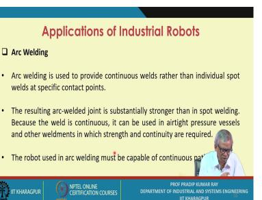
Arc welding is used to provide continuous welds rather than individual spot welds at specific contact points.
