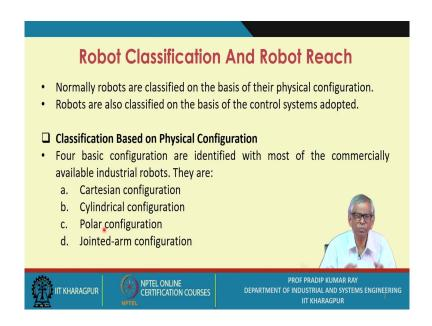
Normally robots are classified on the basis of their physical configuration. Robots are also classified on the basis of the control systems adopted.
