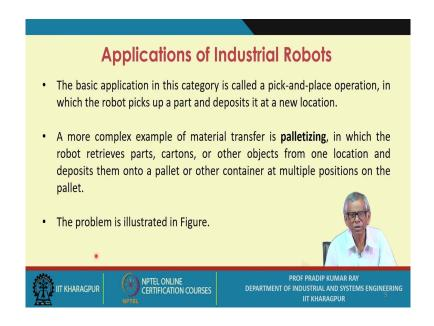
The basic application in this category is called a pick-and-place operation, in which the robot picks up a part and deposits it at a new location. A more complex example of material transfer is **palletizing**, in which the robot retrieves parts, cartons, or other objects from one location and deposits them onto a pallet or other container at multiple positions on the pallet. The problem is illustrated in Figure 8.11.
