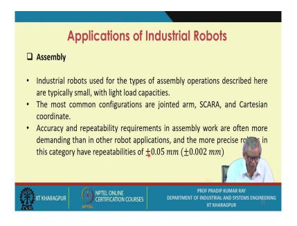
The robots are used assembly operations. Industrial robots used for the types of assembly operations described here are typically small, with light load capacities. The most common configurations are jointed arm, SCARA, and Cartesian coordinate. Accuracy and repeatability requirements in assembly work are often more demanding than in other robot applications, and the more precise robots in this category have repeatabilities of
