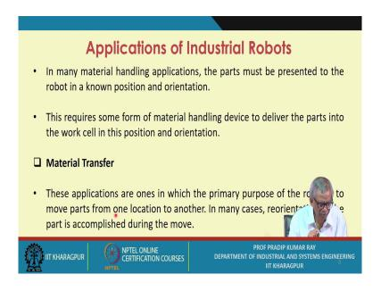
In many material handling applications, the parts must be presented to the robot in a known position and orientation. If there has to be part programming. In an automated system, this location should be known. This requires some form of material handling device to deliver the parts into the work cell in this position and orientation.
