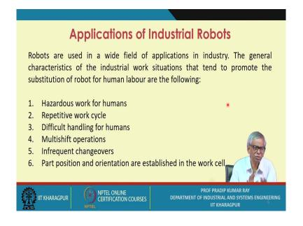
Robots are used in a wide field of applications in industry. The general characteristics of the industrial work situations that tend to promote the substitution of robot for human labour are the following:
