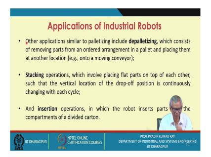
Now, other applications similar to palletizing include depalletizing, which consists of removing parts from an ordered arrangement in a pallet and placing them at another location (e.g., onto a moving conveyor);
