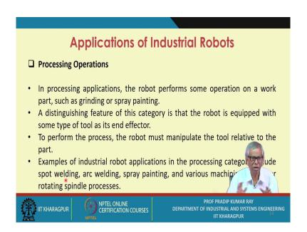
In processing applications, the robot performs some operation on a work part, such as grinding or spray painting. A distinguishing feature of this category is that the robot is equipped with some type of tool as its end effector. To perform the process, the robot must manipulate the tool relative to the part. Examples of industrial robot applications in the processing category include spot welding, arc welding, spray painting, and various machining and other rotating spindle processes.
