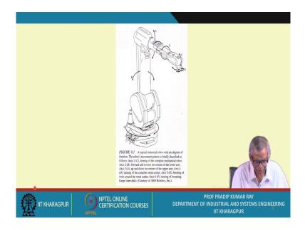
This is the base. This is the lower arm, this is the upper arm, and there is the end effector, there is a wrist. You have the axis C, axis B, axis A, axis D, and axis E.
