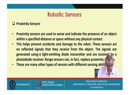
Proximity sensors are used to sense and indicate the presence of an object within a specified distance or space without any physical contact
