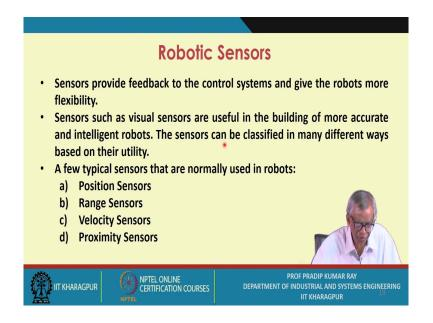
There are four kinds of the sensors; position sensors, range sensors, velocity sensors, proximity sensors.
