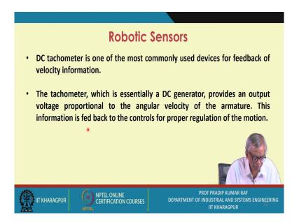
The DC techometer is one of the most commonly used devices for feedback of velocity information. The techometer, which is essentially a DC generator, provides an output voltage proportional to the angular velocity of the armature. This information is fed back to the controls for proper regulation of the motion.
