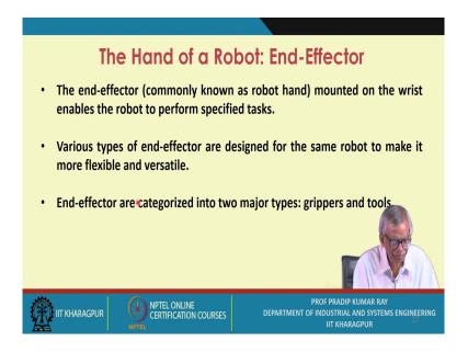
The end-effector (commonly known as robot hand) mounted on the wrist enables the robot to perform specified tasks.
