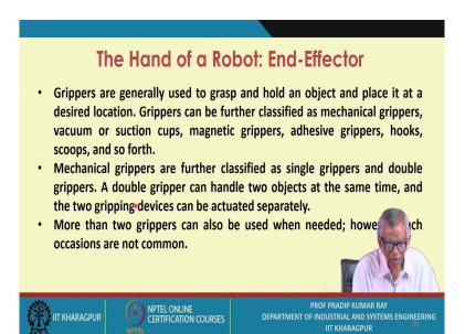
Grippers are generally used to grasp and hold an object and place it at a desired location. Grippers can be further classified as mechanical grippers, vacuum or suction cups, magnetic grippers, adhesive grippers, hooks, scoops, and so forth.
