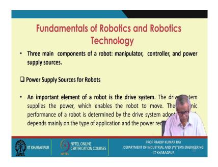
There are three main components of robot, first one is the manipulator, the second one is the controller, and the third one is the power supply sources.
