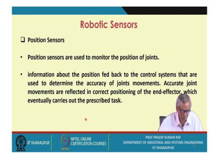
Position sensors are used to monitor the position of joints. Information about the position fed back to the control systems that are used to determine the accuracy of joints movements.
