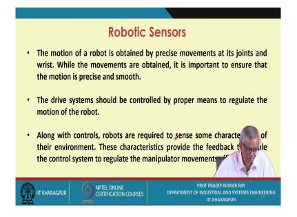
The motion of a robot is obtained by precise movements at its joints and wrist. While the movements are obtained, it is important to ensure that the motion is precise and smooth.
