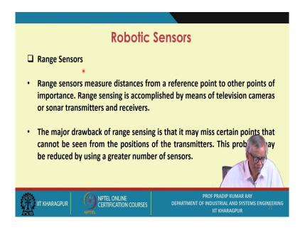
Range sensors measure distances from a reference point to other points of importance. Range sensing is accomplished by means of television cameras or sonar transmitters and receivers. The major drawback of range sensing is that it may miss certain points that cannot be seen from the positions of the transmitters. This problem may be reduced by using a greater number of sensors.
