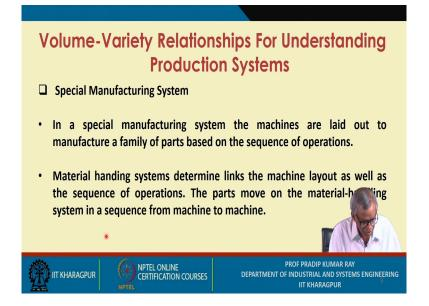
In a special manufacturing system, the machines are laid out to manufacture a family of parts based on the sequence of operations means, is a combination of not only one transfer line, but the several production lines or the transfer line or assembly lines, and from each assembly line the standard product is coming out.
