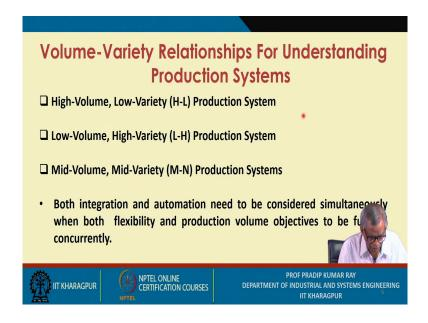
First one is the high-volume low-variety production system; next one is the low-volume high-variety production system, third one mid-volume mid-variety production system. And this is also the classified under three specific types within CIM framework.
