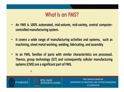
An FMS is an automated, mid-volume, mid-variety, central computer-controlled manufacturing system. It covers a wide spectrum of manufacturing activities such as machining, sheet metal working, welding, fabricating, and assembly. In an FMS, families of
