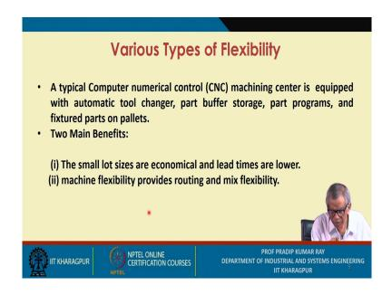
Computer numerical control (CNC) machining centers are normally equipped with automatic tool changer, part buffer storage, part programs, and fixtured parts on pallets.
