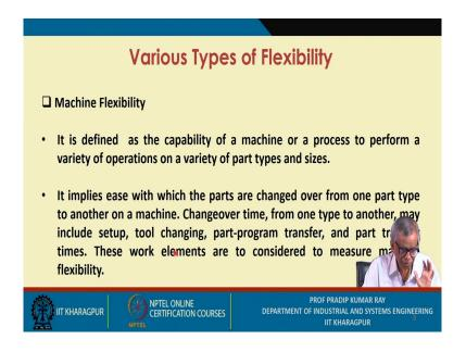
First one is the machine flexibility. It is a capability or ability of a machine or a process to perform variety of operations or a variety of part types and sizes, it implies ease with which the parts are changed over from one part type to another on a machine.
