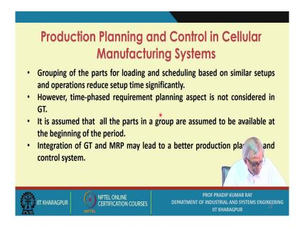
The grouping of the parts for loading and scheduling based on similar setups and operations will reduce setup time. On the other hand, the time-phased requirement planning aspect is not considered in GT. That is, all the parts in a group are assumed to be available at the beginning of the period. Integration of GT and MRP will lead to a better production planning and control system.
