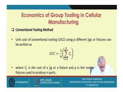
If it is a conventional tooling method, The unit cost of conventional tooling (UCC) using p different jigs or fixtures can be written as
