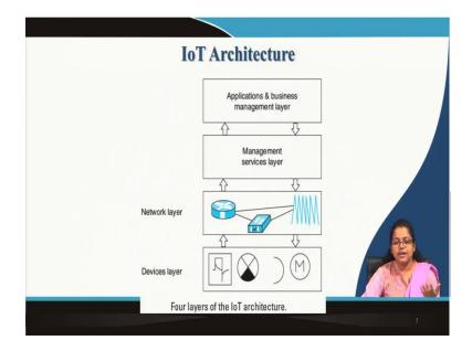
Now, coming to the IoT architecture, this is a very simple you know explanation of what the IoT architecture is without getting into the technical details. So, the IoT architecture comprises of 4 layers, the first layer is called the devices layer that you see here. The devices layer has sensors and actuators. So, the sensors of course, collect data we do have two categories of sensors we have already discussed simple sensors and smart sensors.
