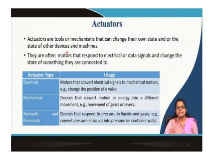
Moving on, actuators so along with sensors comes the term actuators. Actuators are tools or mechanisms, that can change their own state and or the state of other devices and machines. So, they are often motors that respond to electrical or data signals and change the state of something they are connected to.
