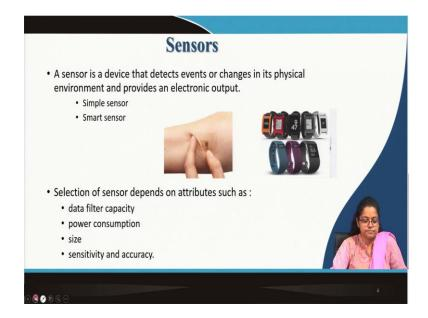
So, we have just spoken about sensors. What are sensors? A sensor is a device that detects events or changes in its physical environment and provides an electronic output. So, here you see you know there are two categories of sensors simple sensors and smart sensors.
