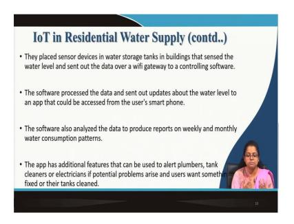
So, let us see what the company has done, they placed sensor devices in water storage tanks in buildings, that sensed the water level and sent out data over a Wi-Fi gateway to a controlling software. Again you will be able to relate to the architecture, that we have discussed in the previous slide.
