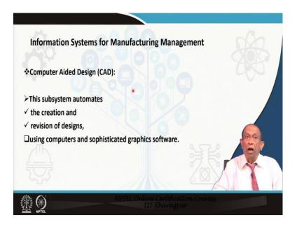
Now we come on to the topic of computer aided design, this is also embedded or interfaced with manufacturing management information systems. The computer aided design subsystem basically automates the creation and revision of product designs using computers and sophisticated graphics software.
