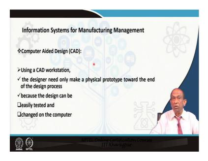
So, using a CAD workstation the designer need only make a physical prototype towards the end of the design process, because the design can be easily tested and changed on the computer.
