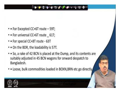
On Indian Railways the permissible carrying capacity of a BCN is, for expected CC plus 6 ton route 59 tons. For universal carrying capacity 6T route is 61 tons, for special 63 tons on the Bangladesh railways load is 57 tons, this is exactly what I was telling when we were discussing road transport in the previous week. Previous to previous week see the carrying capacity differs.
